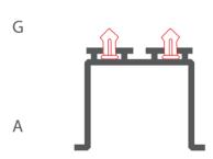
**4.** Mount the LED strip (E), insert the cover (F), insert the end cap (B).
